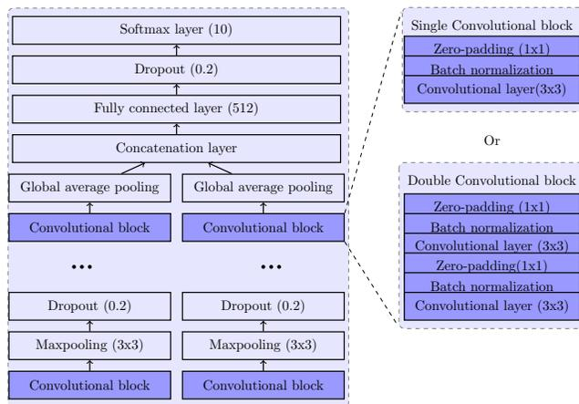
Figure 2: Illustration of the MI-CNN, single and double convolutional blocks.
