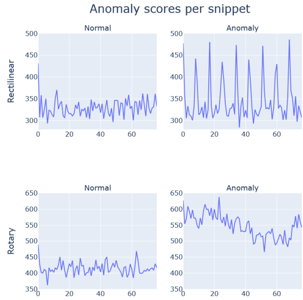
Figure 2: This figure shows the anomaly scores computed by one of our flow based models for some representative examples for a rectilinearly moving machine (valve: normal_id_02_00000038 , anomaly_id_02_00000003 ) and a rotary machine (fan: normal_id_06_00000043 , anomaly_id_06_00000010 ).
