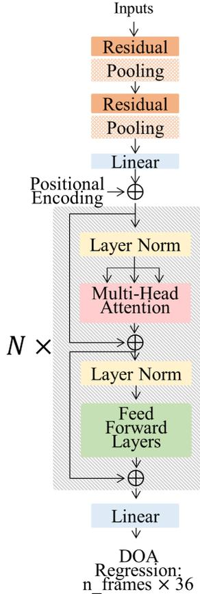
Figure 2: Transformer Encoder for SELD.
