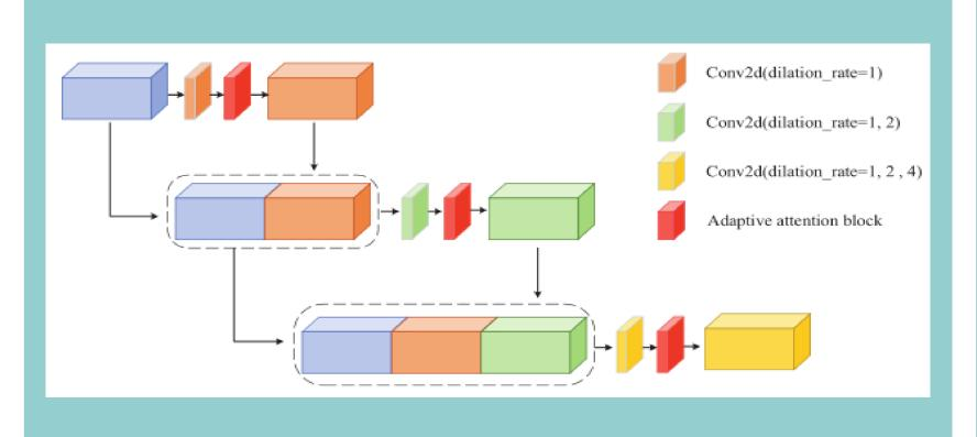
The maximum dilation rate in the last layer depends on the size of the input feature.
