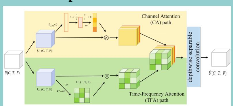
The parallel structure is applied in adaptive attention block which adaptive mitigates interference between the channel-wise and time-frequency-wise by exploring two different branches.
