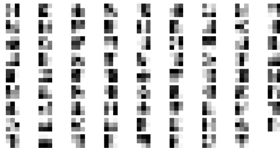
Figure 5: An illustration of the 3 \times 3 filter weights W of the first CNN layer.
