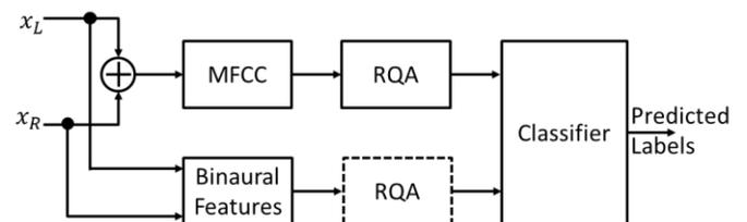
Figure 1: Block diagram of the scene classification system
