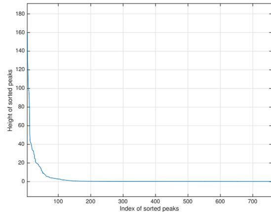
Figure 3: Height of sorted peaks of sequence  $s$ . A “knee” can be observed.
