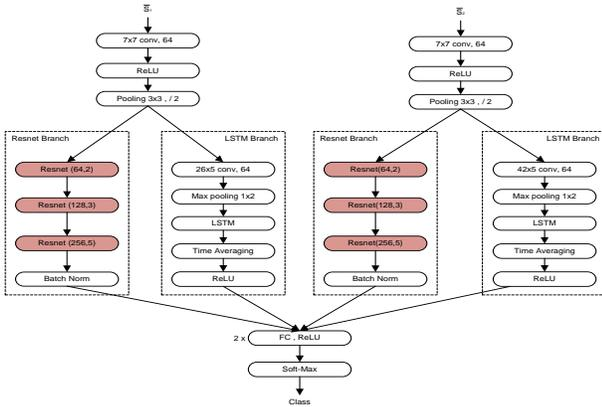
Fig. 3. Schematic description of the proposed neural network architecture.
