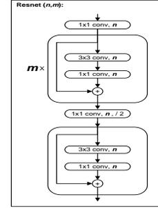
Fig. 4. Description of the building block of the RESNET branch detailing the blocks marked in color in Fig. 3.
