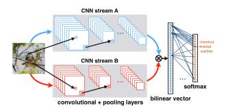
In our model, we fully shared the parameters of CNN A and CNN B, it also means that we just use one CNN and use the matrix outer product to CNN's output with its transposition. We use ResNet34 as convolutional. The shape of input data is 3x60x60, after ResNet34 which cut out the pooling layer and fully connection layers, we get the shape of [512 x 2 x 2], then we reshape it to
