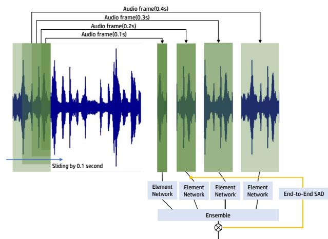
Figure 1: A block diagram for the proposed system.
