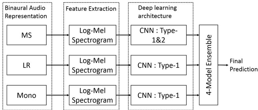
Figure 1: Our overall solution framework consisting of binaural audio representation, feature extraction steps, multiple CNNs & model ensembling for final prediction of the acoustic scene.
