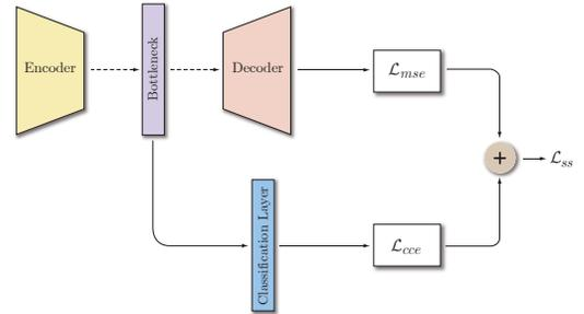
Figure 2: Semi-supervised autoencoder architecture
