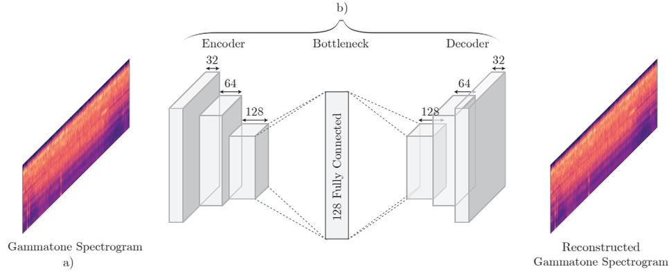
Figure 1: Full framework for ASD based on a Convolutional Autoencoder. Step a) shows the chosen audio representation and step b) the designed autoencoder architecture. The numbers indicate the number of filters in each convolutional block.
