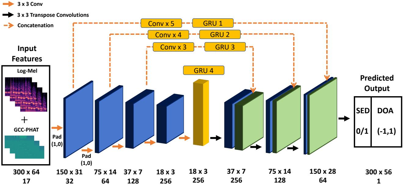
Figure 1: Fully convolutional architecture with skip conv-GRU layers for SELD
