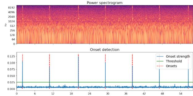
Figure 2: Tick onset detection in valve sounds. Comparison of power spectrogram calculated from one sample with onset strength envelope.
