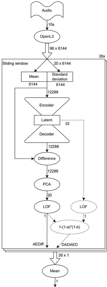
Figure 1: Scheme of the anomaly detection model. The dotted part shows how the AEDiff model is extended by a second anomaly detector – this extension is called DADAED (Double Anomaly Detector AEDiff). Numbers show the dimensions of vectors.
