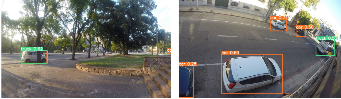
Figure 3: Example of mislabelled vehicles by YOLO.
